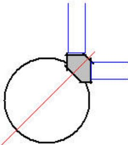
Cut the top of the poles so that shear the loads are embedded. Bolt through the post at 3" end distance and 9" centers to make the bracket integral with the posts themselves.
